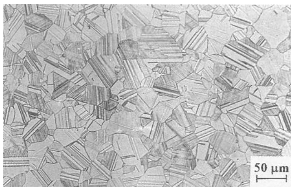
Figure 1 - Microstructure of Co-27Cr-5Mo-0.05C alloy annealed 2 hours at 1100 °C.
