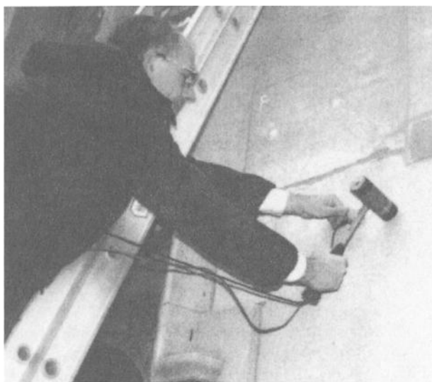
FIG. 5— Impulse Response Testing.
