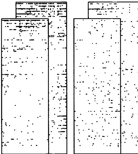
Figure 7 - Identifying deficiencies on separate layers in Autocad permits selective printing in order to see patterns or proximity of deficiencies. The dots on the image at left show an increased density of cracks along the top and right side of the building, while the spalls shown in the image at right are generally more sporadic.
