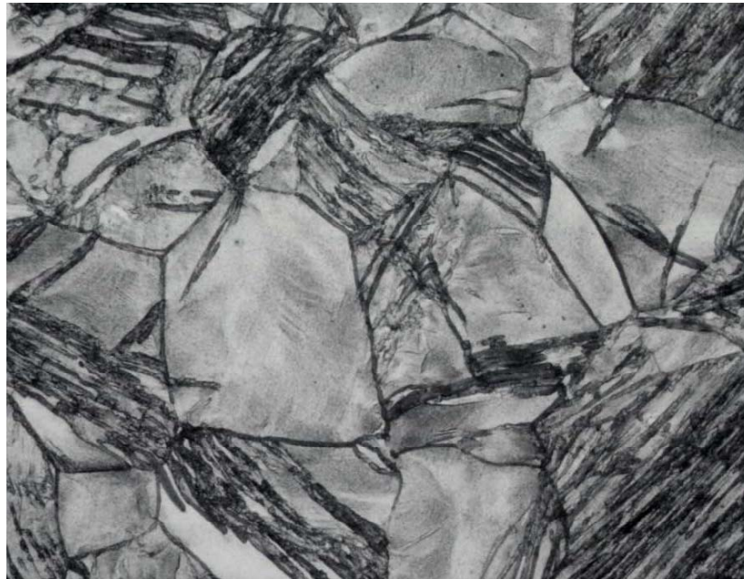
FIG. 10— Ti-15Mo that has been 40 % cold drawn and aged reveals uniform alpha precipitation within the microstructure (500 \times ).
