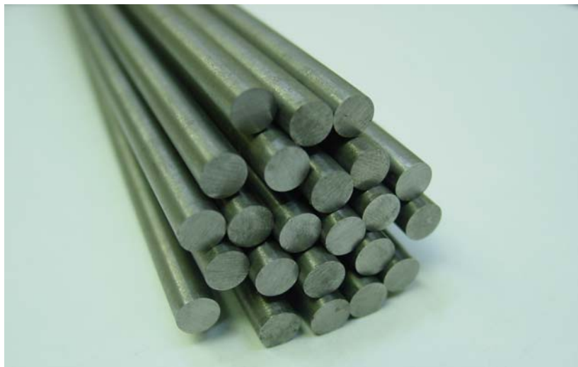
FIG. 4—High strength 5.4 mm diameter Ti-15Mo 40 % cold drawn, fully heat-treated rod stock.
