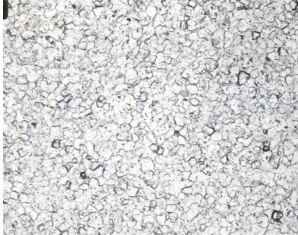
FIG. 1— Representative microstructure for cpTi showing equiaxed alpha grains. Original magnification = 200 \times .
