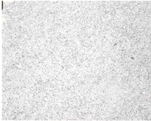
FIG. 2— Representative microstructure for Ti64 showing dual phase alpha-beta grains. Alpha regions are light and intergranular beta regions are dark. Original magnification = 200 \times .
