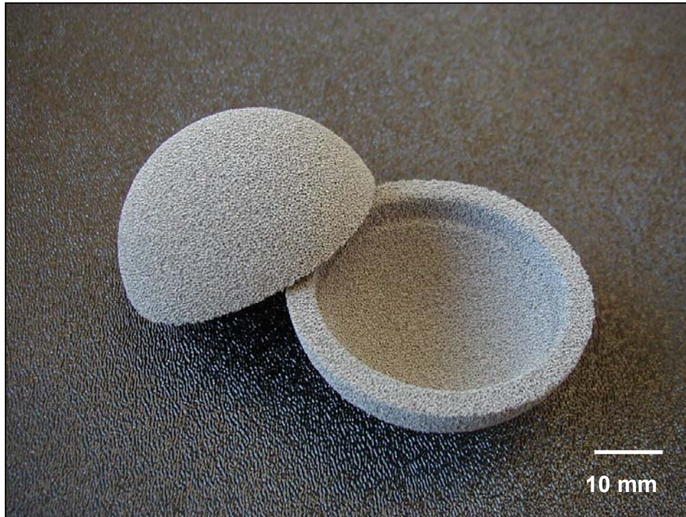
FIG. 1— Tantalum foam acetabular shells 40 mm in diameter.
