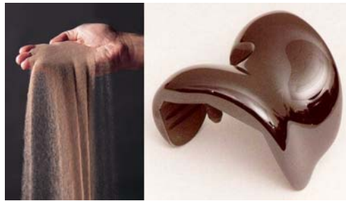
FIG. 1—Zircon sand (left) is the raw material used to make an oxidized zirconium implant (right).
