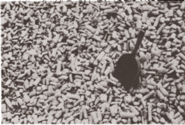
FIG. 11— Flue gas gypsum briquets in storage.
