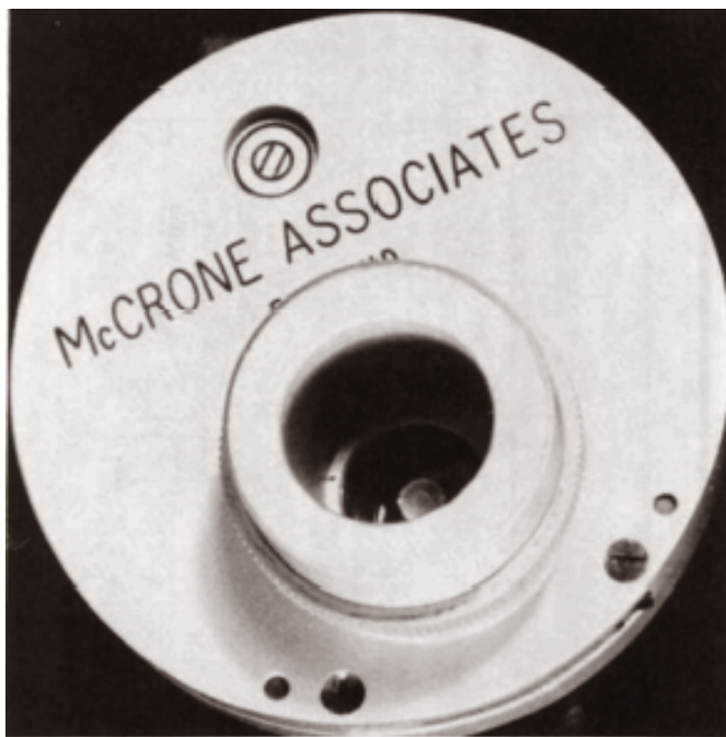
FIG. 12—Dispersion staining devise showing central stop.
